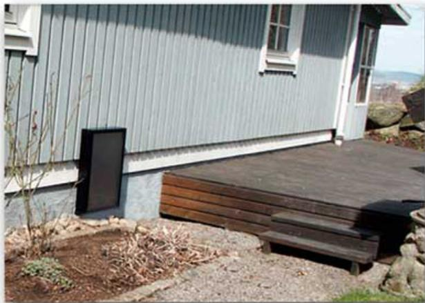
The easiest installation is directly against the wall, with the flextube pushed through existing vent/opening. If the SolarVenti is tilted slightly, it will be more effective than if installed in a vertical position.
